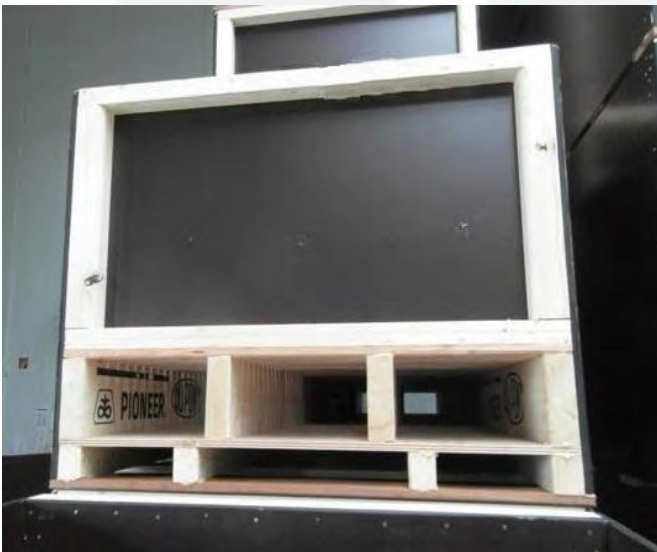
Example drying box with double pallets: ventilation and transport. Box with plywood with coating.
