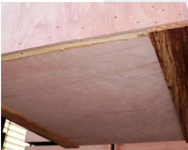
Pallet bottom closed by 9mm plywood.
